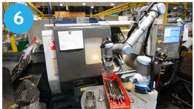
Drops the finished part into a bin.
