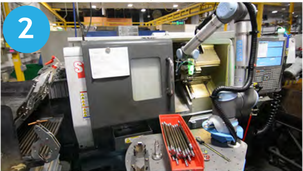
Fits the part into the jig in the CNC lathe.
